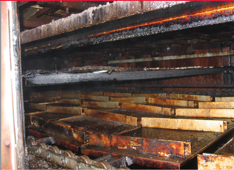
Dryer entrance showing hydrocarbon condensate
