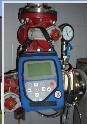
Biogas Flare that produces 2.5 MMBtu/hr of energy that is not being utilized and the associated testing equipment to track methane concentration
